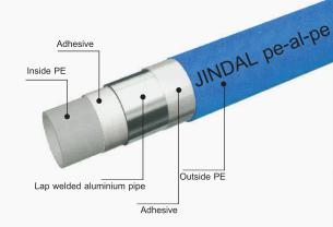
Jindal MLC Pipes consist of an overlapped aluminum core with an inner and outer layer of polyethylene (PE). All the layers are permanently bonded together by intermediate adhesive layers. The aluminum thickness of Jindal MLC pipes has been selected to meet compressive and flexural strength requirements.
